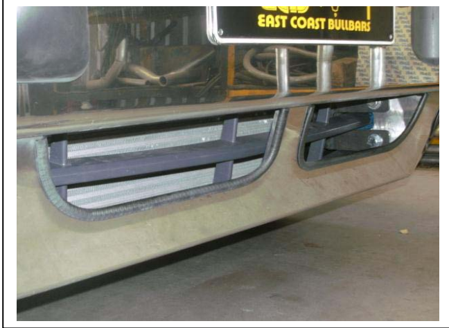
Figure 13: 3mm clip lock on centre skirt
