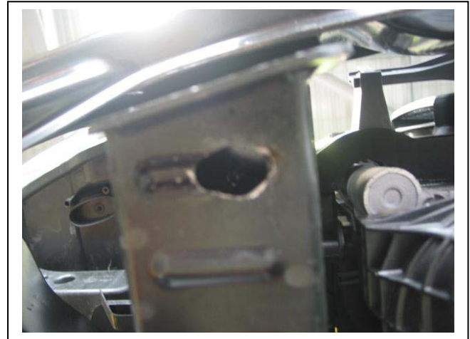
Figure 4: Enlarge hole in underside of chassis rail
