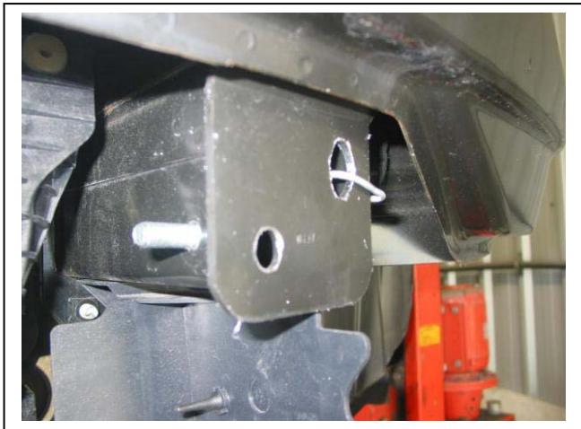
Figure 7: Cut and crimp wire to side of opening
