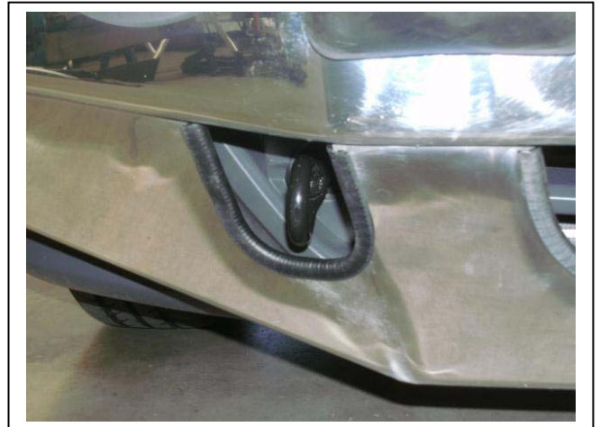
Figure 14: 3mm clip lock on end skirt Drivers side shown (tow hook fitted)
